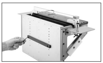
Figure 14. Attaching the miter bar to the jig.
